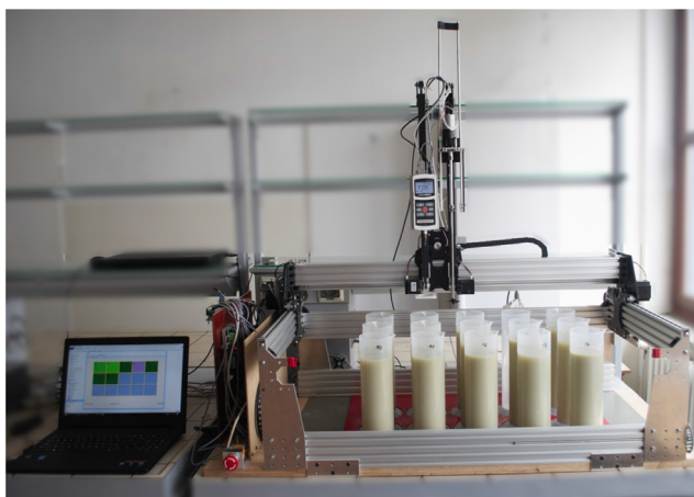
Fig. 1. The device used in the dynamometer method with the integrated x-y sample changer.
